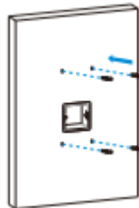
Insert the screw fixing seats into the hole
