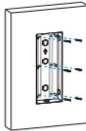
Place the embedded box into the square hole the edges of which align to the wall and make all cables go through the cable hole. Fix the embedded box with 6 TS4x20 screws. Then use cement or non-corrosive structural adhesives to fill the gap between the wall and embedded box
