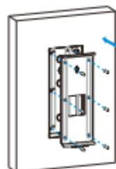
Use six M4X10 screws to fix the flash-mounting bracket on the embedded box.
