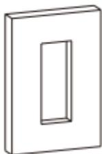
Dig out a square hole (height\*width\*depth=269.5\*122.4\*60.5mm) Note: The size of the hole should be a little bigger than recommended value that can accommodate all cables.
