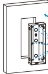
Insert the embedded box into the hole and make sure the cables of the device can route through the cable hole. Then mark the six holes of the wall embedded box on the wall
