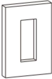
Dig out a square hole (height\* width\*depth=269.5\*122\*4\*60.5 mm)
