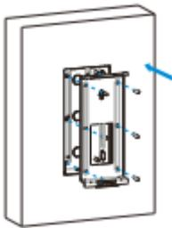
Use six M4x10 screws to fix the flash-mounting bracket on the embedded box
