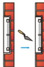
Use cement or non-corrosive structural adhesives to fill the gap between the wall and embedded box. Wait the adhesives material desiccation, go to the next step
