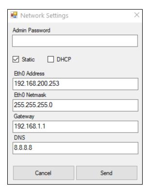
From here, you are able to directly send the new network settings to the device.
