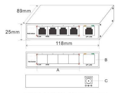
A. 4\*PoE Ports B. Uplink Port C. DC Power Input Port
